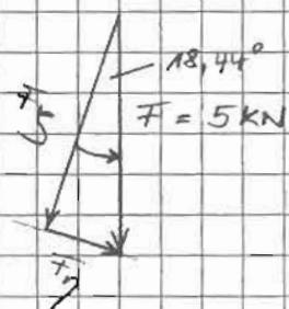
$$F_y = -5 \text{ kN} \cdot \sin 18,44^\circ = -1,582 \text{ kN}$$
