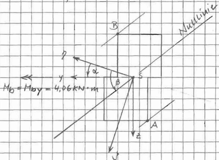
$$M_{by} = M_b \cdot \cos \alpha = 4,06 \text{ kN} \cdot \text{m} \cdot \cos(18,44^\circ) = 3,852 \text{ kN} \cdot \text{m}$$
