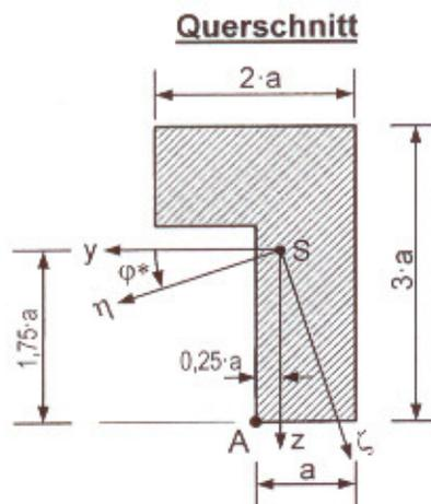
$$\varphi^* = 18,43^\circ; \quad I_\eta = \frac{10}{3} \cdot a^4; \quad I_\zeta = \frac{25}{30} \cdot a^4$$
