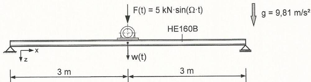
Profil HE160 B:  $\rho = 42,6 \text{ kg/m}$ ;  $I_y = 2490 \text{ cm}^4$ ;  $W_{by} = 311 \text{ cm}^3$
