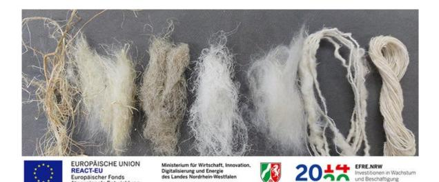
Development of an innovative process chain for processing german hemp and recycled wool into textile products
