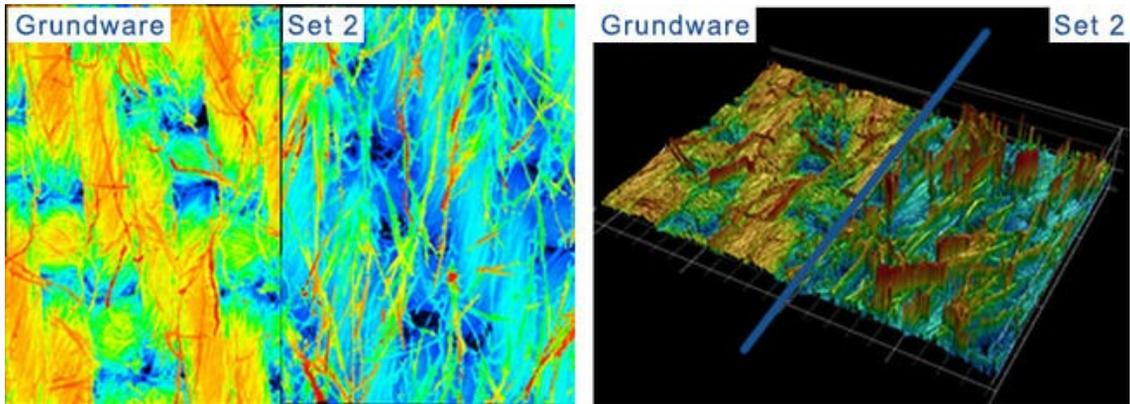
**HapTex 4.0 - Development of a roughness-guided continuous quality and surface control in the dry finishing of textiles by means of a haptic sensor that can be widely used in the textile industry. Partial project: Realization of a new evaluation scale for the grip assessment of textiles based on measurement data from a haptic sensor for implementation in virtual product development processes**
